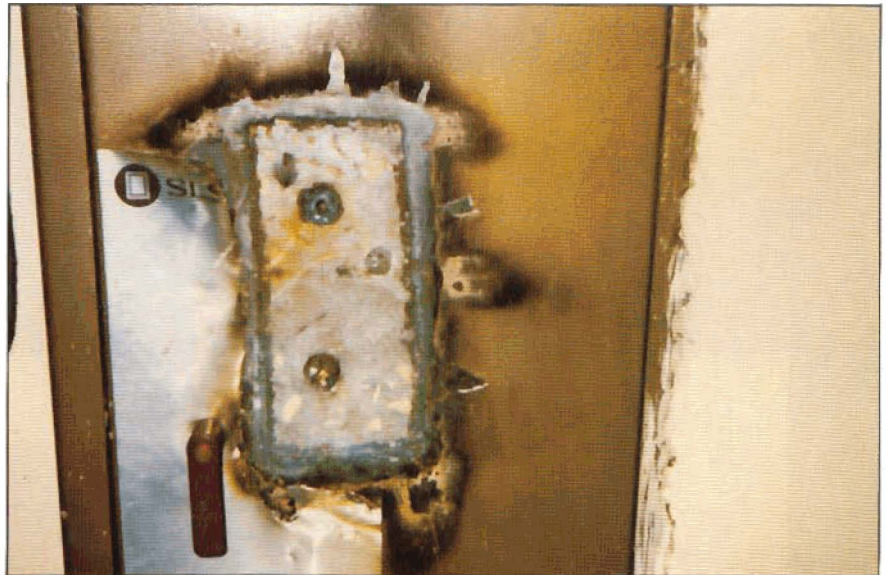
Unsuccessful Torch and Tool Attack on the SLS Continental Mark IV at a Jeweller's shop in Malta.
