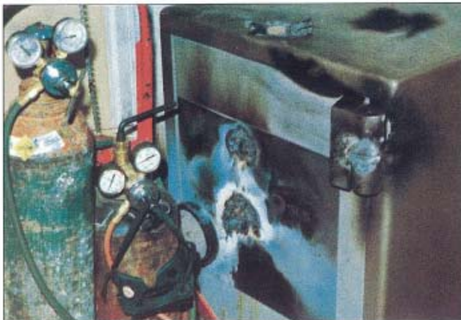
Another Criminal Failure on an SLS TRTL 30 x 6 Safe in the USA.
